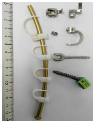
Figure 2. Prototypes of rib hooks, spinal hooks and screws to assemble to the GSDyn.
