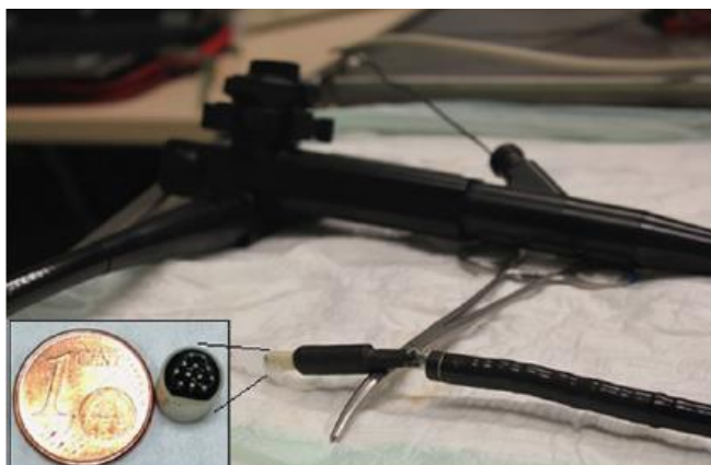
Figure 1. Picture of the developed sensor array inserted in a gastroendoscope. The inset picture shows the size of the array.
