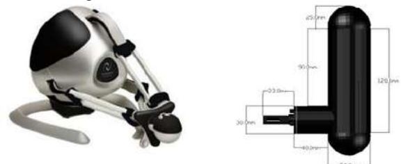
Figure 1. Novint Falcon haptic device and the novel HandGrip designed for Novint Falcon
