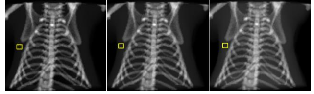
Figure 7. Bone tissue images extracted with the implemented algorithm when the soft tissue equivalent material of the calibration phantom is water (left), plastic A-150 (center) and PMMA (right). The yellow square indicates the measured ROI: 0.7(left), 1.16 (center) and 1.9 (right).
