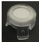
Figure 2. Cell crown with PCL 10% mesh where HTMC are seeded
