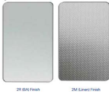
Figure 1. Images of the non-textured reference (2R BA Finish) and textured (2M Linen Finish) collectors used for the comparative study.
