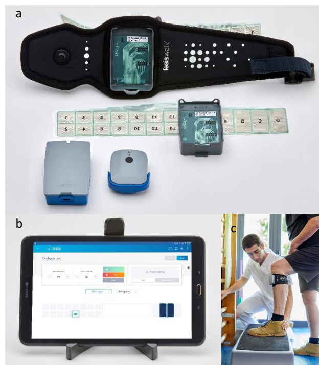
Figure 1. The Fesia Walk system (Fesia Technology, Donostia – San Sebastián, Spain). a Stimulation unit, garment, multi-field electrode and wireless sensor. b Tablet PC with software application. c Neurorehabilitation with FES.
