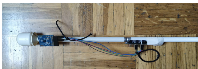
Fig 1. Long cane (117 cm) with the incorporation of the IMU sensor and Arduino MKR1010 for testing.
