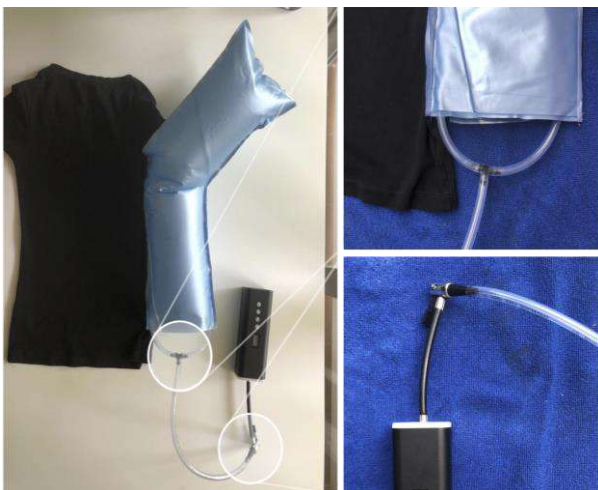
Figure 5. At the left, inflated exoskeleton sewn to T-shirt. At the right, T junction and connection to air compressor.
