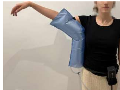
Figure 7. Patient wearing inflated exoskeleton
