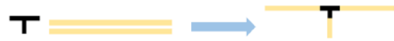
Figure 4. T junction. The two plastic tubes are joined in a single tube using a T junction.
