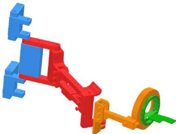
Figure 1. 3D-printed based passive upper-limb exoskeleton assembly. Segments: shoulder/back in blue, arm in red, forearm in orange, and hand in green
