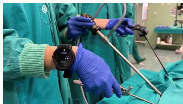
Figure 1. Experimental setup: Surgeons wearing a smartwatch on their dominant hand in order to register acceleration data from the smartwatch's IMU
