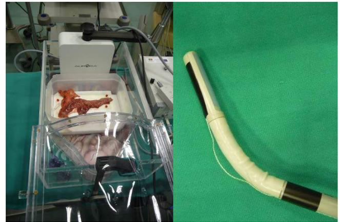
**Figura 2.** left) Experimental set showing the porcine pancreas, fiducial markers as red spheres and the Aurora electromagnetic tracking system; right) 6DOF sensor attached to the LUS probe.
