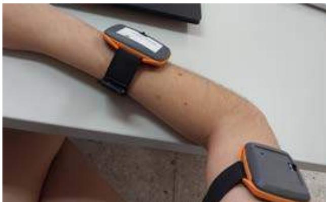
**Figure 4.** Position of the inertial sensors on upper arm and forearm, which are also used as markers for Kinovea analysis
