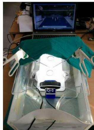
**Figura 3.** Testing setting. The KTS box is placed inside the SIMULAP IC-05 box trainer and covered with a surgical drape. The camera is used to track laparoscopic instruments, and occupies a fixed position
