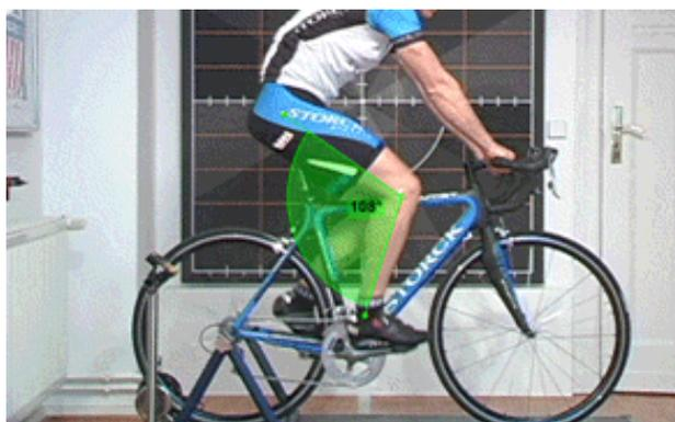
Figure 1. Example of range of motion estimated using the Kinovea software
