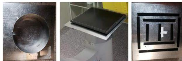
Figure 6. Part of the holder that is introduced in the C-arm detector (left). Flat panel fixed to the C-arm. (middle) Part of the holder that is attached to the flat panel (right)
