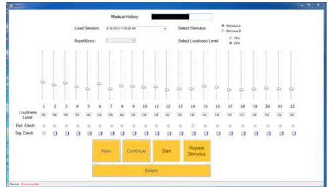
**Figure 4.** Loudness Balance view. After selecting which stimulus and at which percentage of the DR to work with, this test serves to level the intensity of all electrode through a confluence method.
