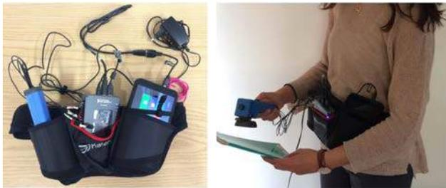
Figure 4. Final B-HelpR prototype's appearance and demonstration of how to wear it.
